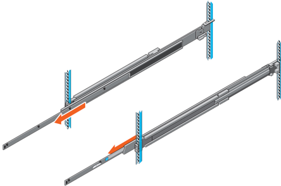
Figure 25. Pull out inner rail
