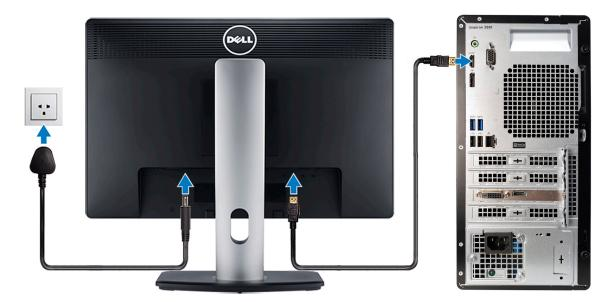
(i) **NOTE:** If you ordered your computer with a discrete graphics card, the HDMI, VGA and the DisplayPort on the back panel of your computer are covered. Connect the display to the discrete graphics card.
