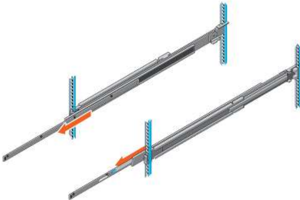
Figure 27. Pull out inner rail
