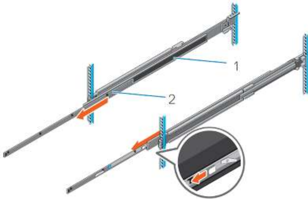
Figure 30. Pull out the intermediate rail
