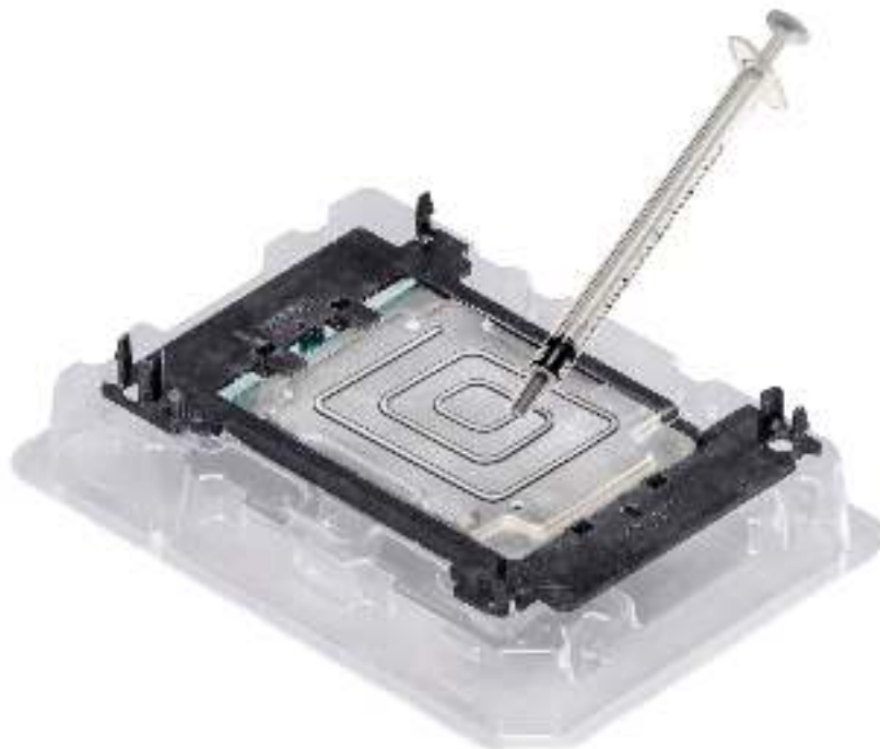
Figure 17. Applying thermal grease on top of the processor
