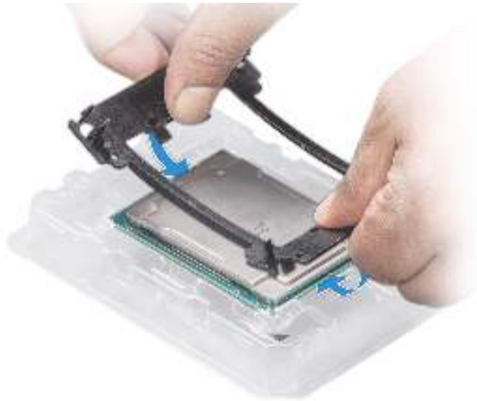
Figure 16. Installing the processor bracket
