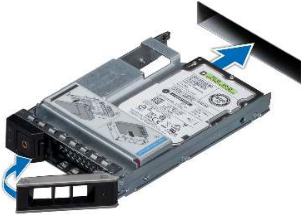
Figure 14. Installing hard drive
