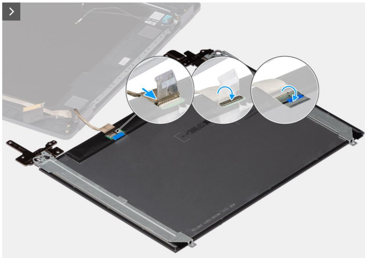
Figure 79. Installing the display-panel assembly
